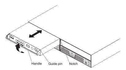
Figure 38. Removing a controller
